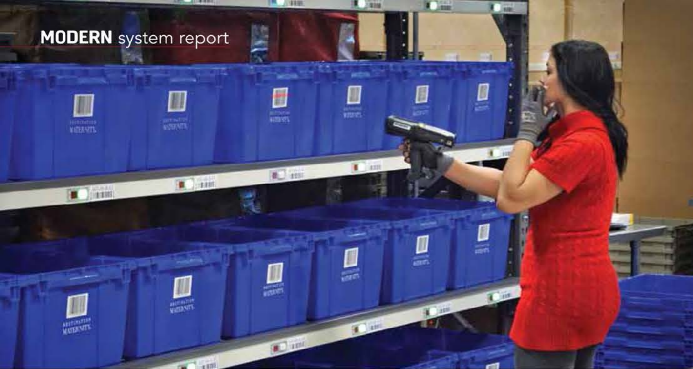
Once items are sorted on the bomb-bay unit sorter, multi-line, store and wholesale orders are completed in a put wall area with more than 2,000 lights.
