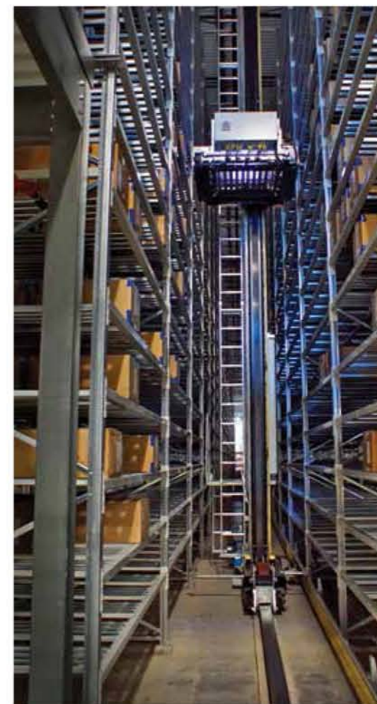
Destination Maternity makes the most of its storage space with a mini-load AS/RS (shown) for cases and totes and a shuttle that manages 26,000 SKUs.
